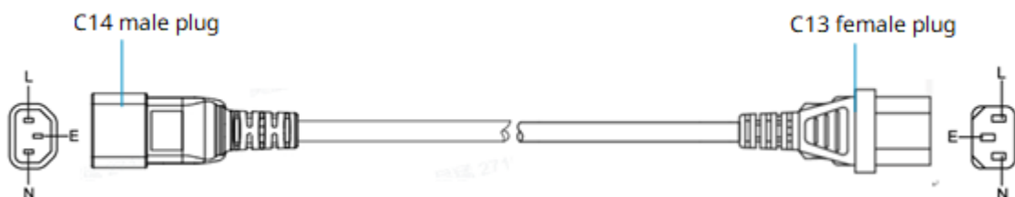
Figure 1-18 AC Power Cord Structure
