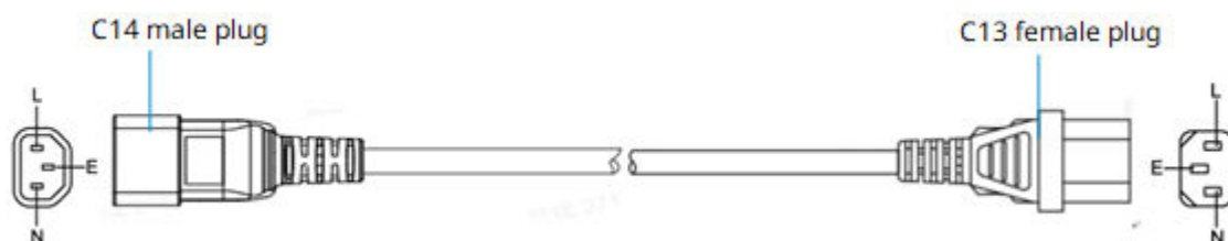
Figure 1-10 AC Power Cord Structure
