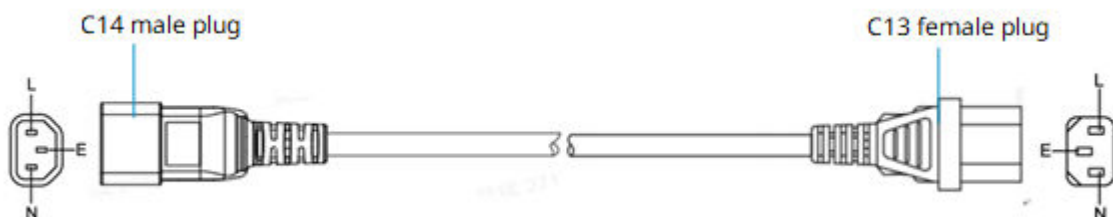
Figure 1-17 AC Power Cord Structure
