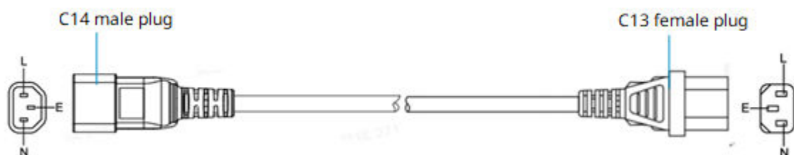
Figure 1-10 AC Power Cord Structure
