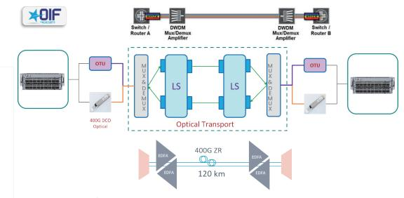
Supporting 400G ZR/ZR+ modules, allowing for up to 120 km long-distance interconnection between IDCs; no intermediate devices; reducing the TCO by 15%–30% when compared with the traditional architecture
